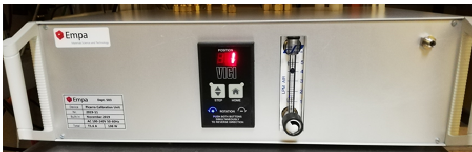
Figure 8: Front view of the calibration unit. The VICI control module allows to manually selecting a specific port. The rotameter allows to check the flow through the inlet line (maintained by an external pump) to the calibration unit. The small excess flow during calibration can be checked at the overflow port on the right.
