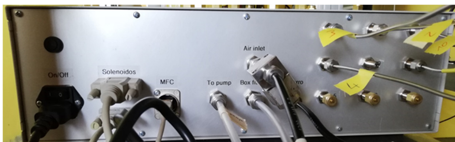
Figure 9: Backside view of the calibration unit. The inlet tube is connected to 'Air inlet' and the external pump is connected to 'To pump'. The port 'To Picarro' is connected with the inlet port of the Picarro analyser with the Nafion dryer (Permapure PD-50T-24SS) in between to dry the sample prior to analysis. Ports 2 to 10 are dedicated for standard gases. The 'MPV' and 'Solenoids' cables are connected to the respective plugs at the backside of the Picarro. 'MFC' (required for the mass flow controller) is connected to a USB port of the analyser. Box flush is connected to the outlet of the Picarro inlet line pump. This ensures that the inside of the box is flushed with ambient air which will minimize contamination in case of a leak in the calibration unit.
