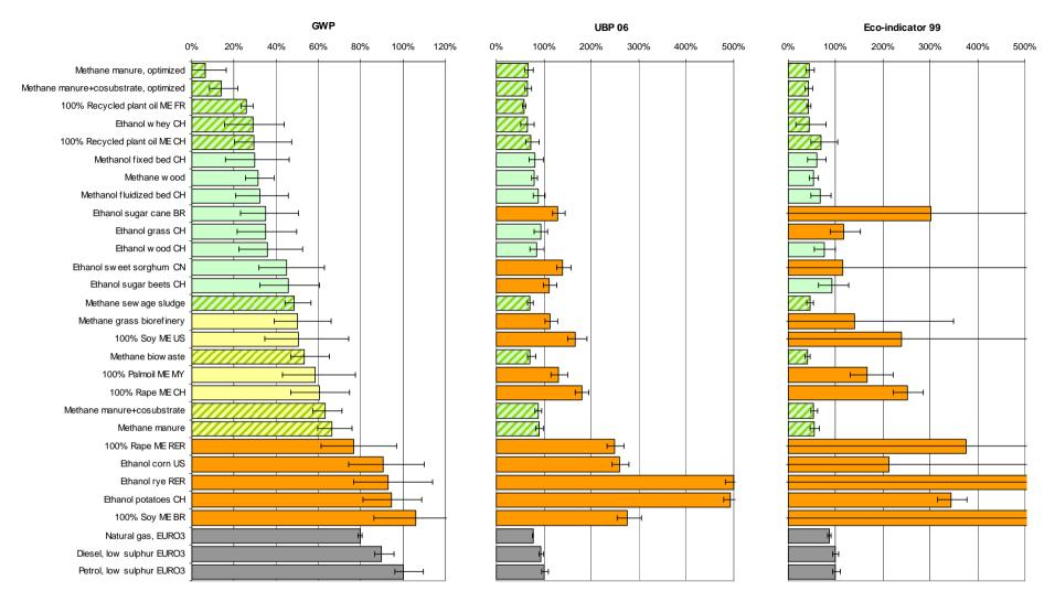
Figure 5 Overall environmental Life Cycle Assessment of all unblended biofuels studied in comparison to fossil reference. GHG emissions reductions of more than 30% are yellow, GHG emissions reductions of less than 30% are red. In other diagrams green = better than reference; red = worse than reference. Cross-hatched fields = production paths from waste materials or residue. Error bar = 2.5 % / 97.5 % percentiles calculated using Monte Carlo simulation.
