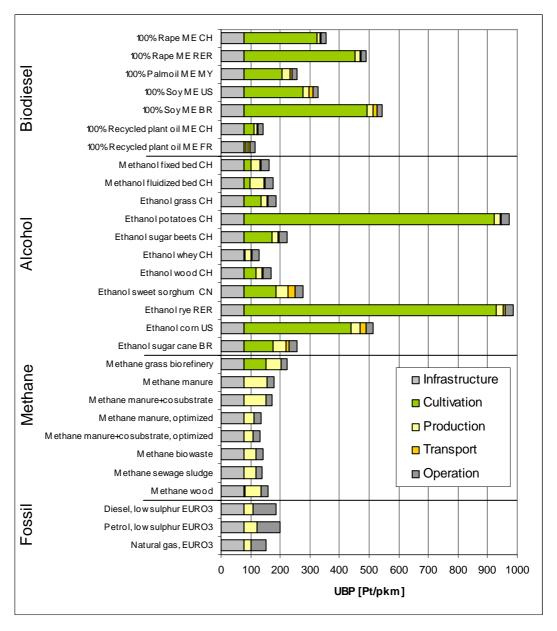
Figure 3 Comparison of aggregated environmental impact (method of ecological scarcity, UBP 06) of bio fuels in comparison with fossil fuels (petrol, diesel and natural gas). The environmental impact is broken down by individual processes of value chain.
