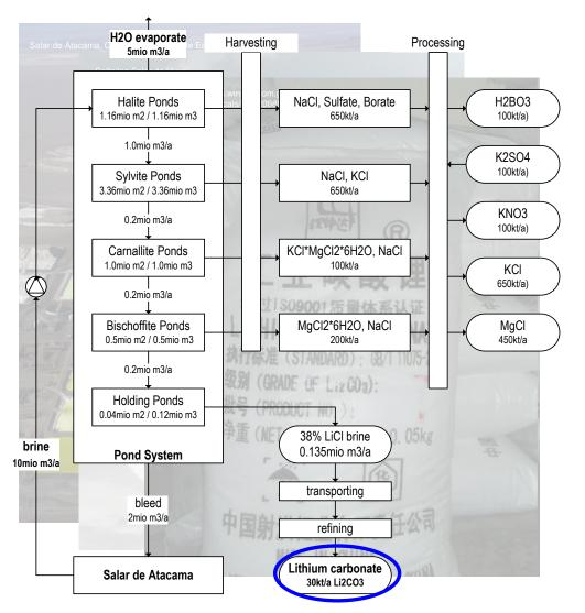
Extraction of lithium carbonate from Atacama (CL), one of the most important worldwide Li2CO3 producers Compilation of numbers and graphics: Empa
