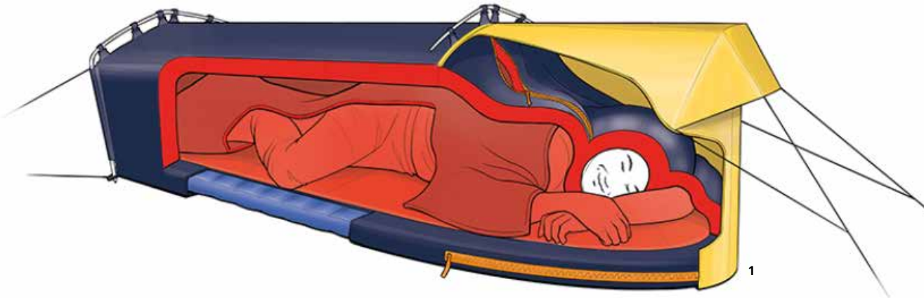
1 Diagram of Polarmond's self-heating bivouac system: sleeping bag (dark blue) with a zip ventilation hole and inlet. (Photo: Polarmond)
