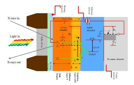
Schematic drawing of a photoelectrochemical cell with a 30 nm thin hematite photoanode (orange), properly wired, in contact with electrolyte (blue), illuminated with visible light, separated by a 100 nm thin membrane from the vacuum environment, and analyzed *in situ* with soft X-rays in the ALS synchrotron.
