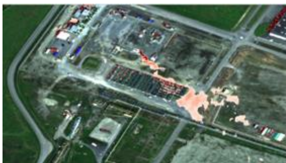
Fig. 1: Example of a detected CH 4 plume from the controlled release experiment in France.
