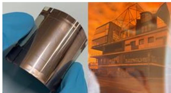
Fig. 1: Photos of a WBG perovskite solar module (left) and a semi-transparent WBG perovskite film (right).
