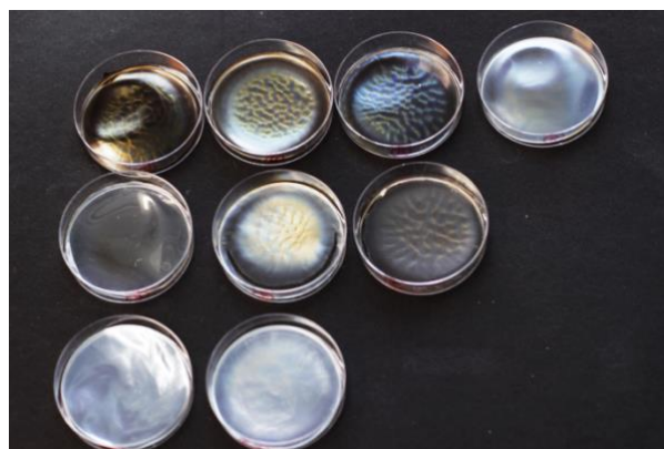
Fig. 1: Structurally coloured film samples after evaporation induced self-assembly of doped CNC films.
