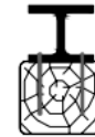
a) Application of pultruded profiles in the compression zone connected by mechanical devices
