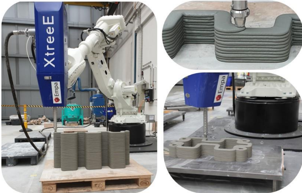
XtreeE 3D-printer robot and digital fabrication of concrete formworks with various shapes.
