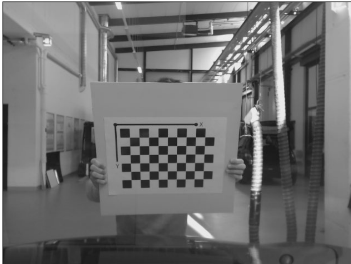
Figure 19: Image from the camera parameter estimation process with a checkerboard.
