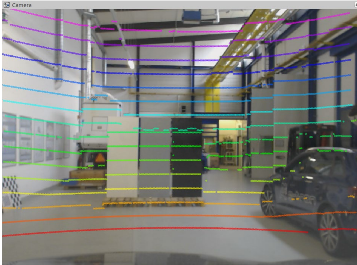
Figure 85: Image of lidar targets at 10m distance with lidar points overlaid.
