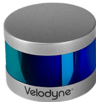
Figure 10: Left: Velodyne (VLP-16-A) LiDAR Puck (Source: [8]). Right: Velodyne installed on the roof.
