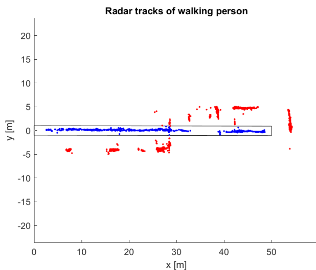
Figure 37: Radar filtering based on region of interest (log 06 from 28.9.2020).
