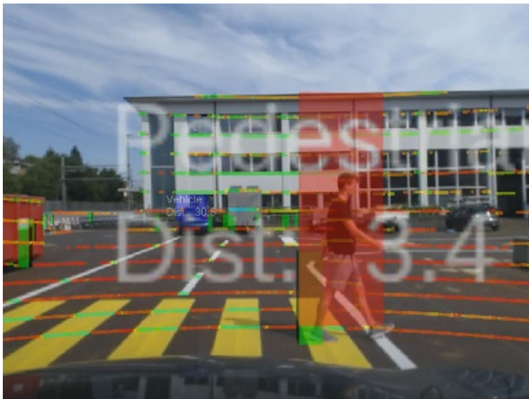
Figure 16: Pedestrian crossing the street. Red box: Mobileye detection. Green cuboid: Radar detection. Colored horizontal points: lidar points with corresponding intensity.
