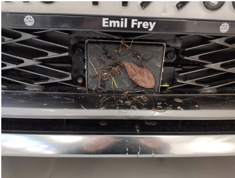
Figure 32: Radar covered with dirt and leaves.
