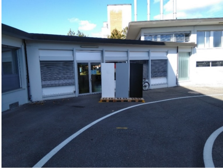
Figure 81: Black, grey and white lidar targets on the test track.
