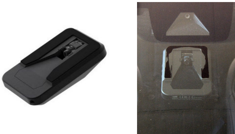
Figure 13: Left: Mobileye 630 camera (Source: [8]). Right: Mobileye Camera Module installed on Lexus.
