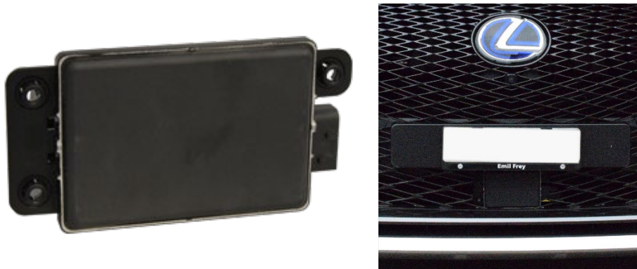
Figure 5: Left: Delphi ESR 2.5 (Source: [8]). Right: Radar fitted into the front grill below the license plate.
