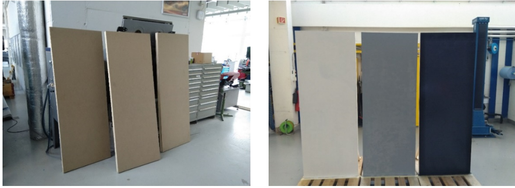
Figure 26: Wood panels for lidar targets.
