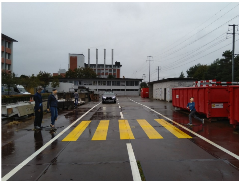
Figure 63: Front straight with AD-vehicle and mannequins during a rain test.
