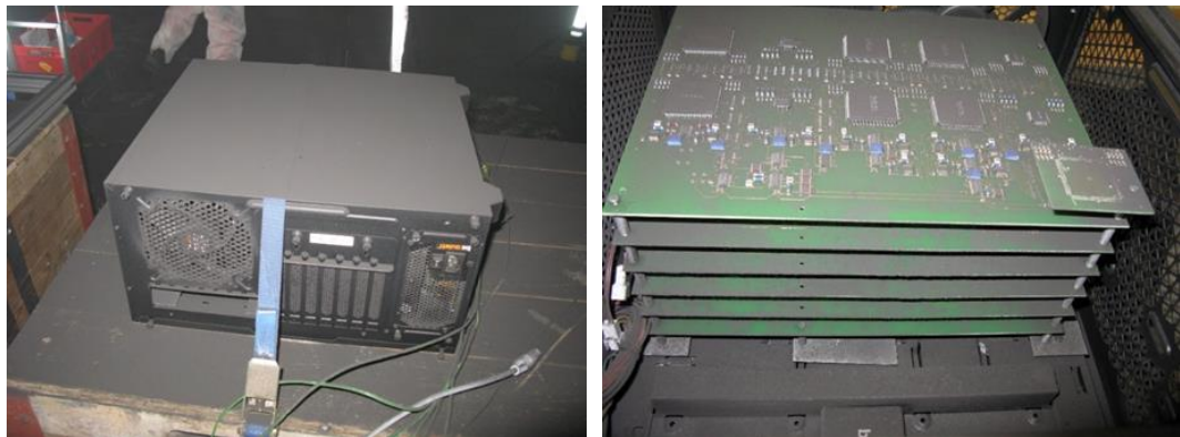
Figure 17 PC housing (left) and circuit boards (right) after fire test
