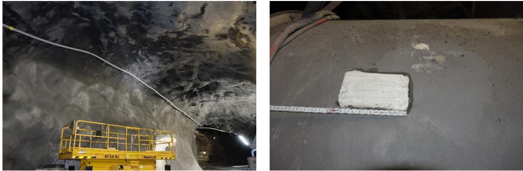
Figure 13 Former test site with black fire soot residue (left) and sampling location SS-1 on the smoke exhaust ventilator housing (right)
