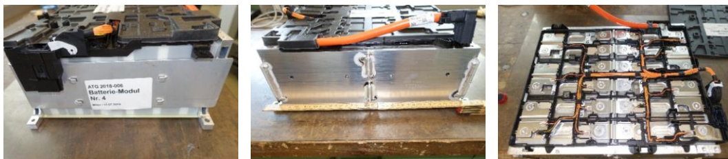
Figure 24 Setup of battery module with investigated components made of plastic and metal
