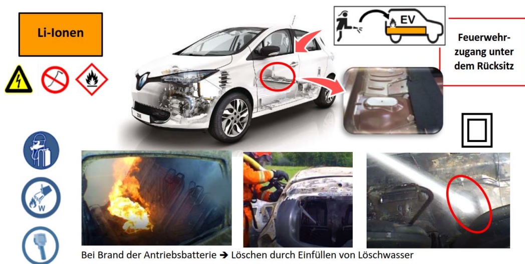
Figure 26 Rescue data sheet for the Renault Zoe 50 stating the specific fire service access point and the recommendation to use water to fight the fire ([69])
