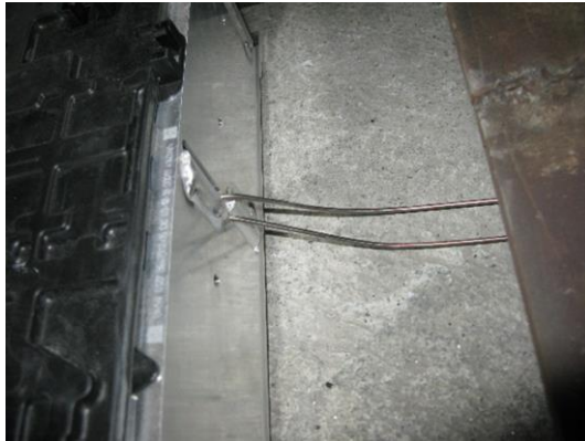
Figure 31 Two sheathed thermocouples with measuring tips in the centre of the battery module
