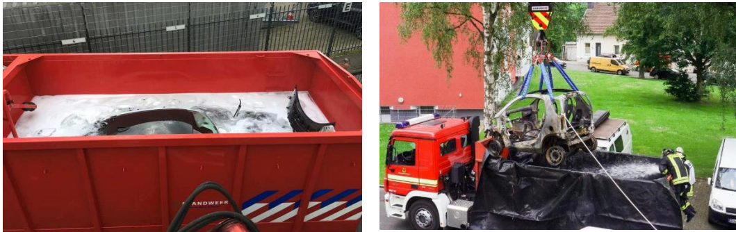
Figure 27 Solutions in current practice for cooling accident-damaged BEV wrecks (for sources see footnotes 4 and 5 )
